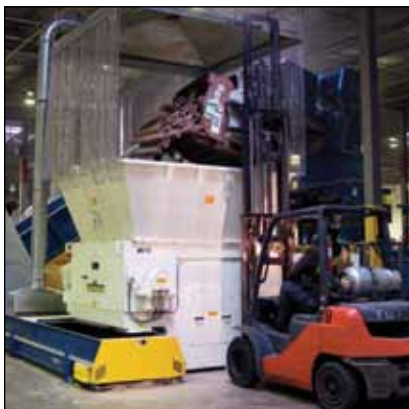
One of Quincy Recycle's Cresswood shredders is loaded with paper cores.
